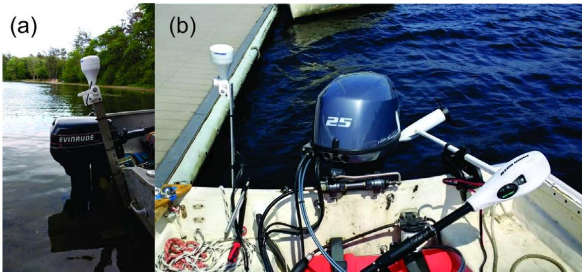
*Figure 2(a): GPS, broadband, and sidescan transducer mast. Note depth markings on mast near transom. (b) Stern of survey vessel, showing clamped mast, outboard, and trolling motor*
