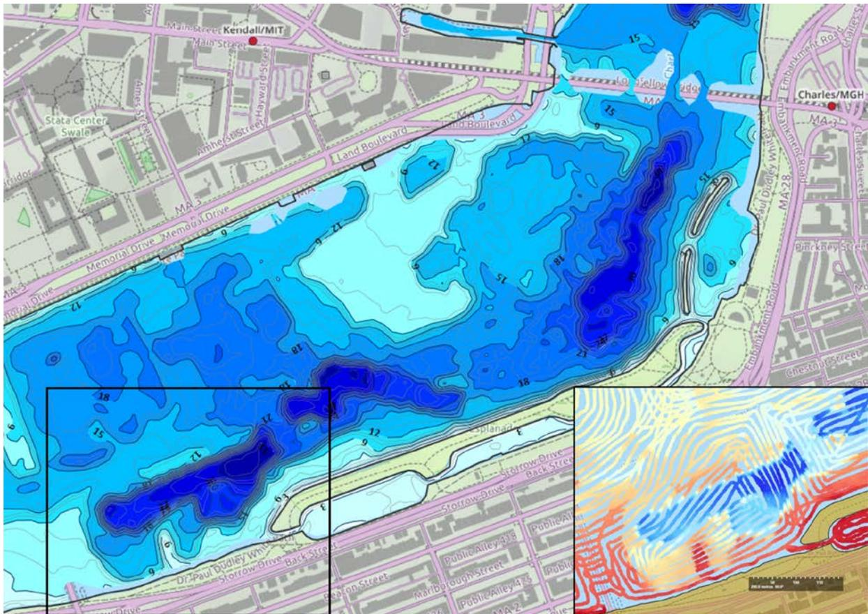
Figure 3: Contour view of chart section in ReefMaster before refinement in ArcMAP. Inset shows detail of survey sonar tracks. Scale bar is 200 m long. Red indicates shallow portions of the track, blue deeper
